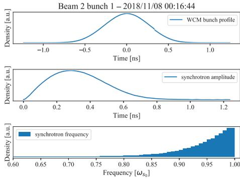
Figure 1: Top: typical bunch profile at flattop, measured by a Wall Current Monitor; Middle: synchrotron amplitude distribution derived from Eq. (4); Bottom: synchrotron frequency distribution derived from Eq. (2).
