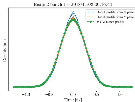
Figure 5: Bunch shapes derived from the Horizontal and Vertical LHC Schottky spectra in a time interval of 100 seconds around WCM measurement.
