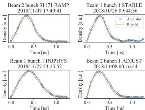
Figure 3: Synchrotron amplitude distributions calculated for different beam modes are shown to follow a Rice distribution. Optimal Rice parameters were found as a result of curve fitting.
