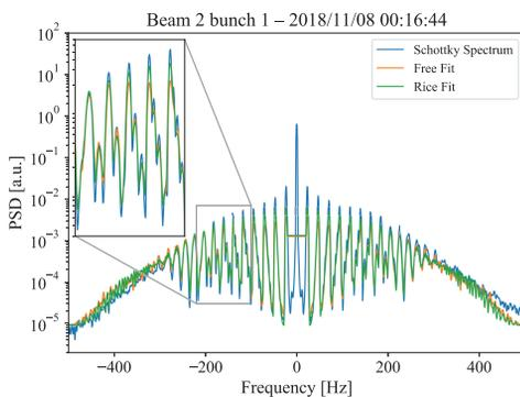
Figure 4: Rice and free fit spectra compared with an experimental Schottky spectrum. There is no fit for the  $p = 0$  satellite, as it adds up coherently and Eq. (9) does not hold.
