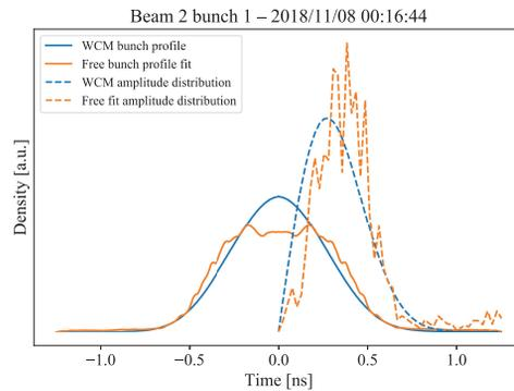
Figure 2: WCM bunch profile and results of bunch profile fitting. Without putting any constraints on the synchrotron amplitude distribution we end up with an exotic bunch shape.
